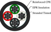
Reinforced CPE Jacket Stranded Tinned Copper Conductor
